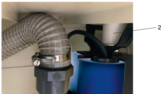
Fig. 17: Correct installation position of cover and pump set
