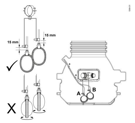
Figure 6: Sanisett float switch installation (\* cable ties)
