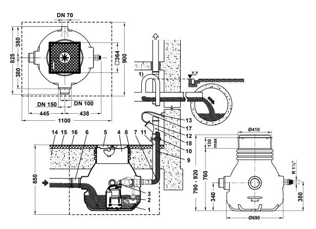
Figure 2: Sanisett installation example and dimensions
