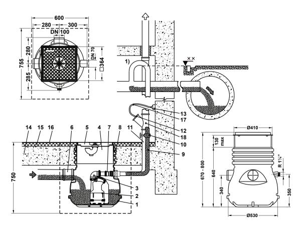
Figure 1: Nirolift installation example and dimensions
