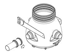
Figure 3: Opening connection ports
