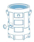
SANIFOS® 280, 610 and 1300 have several drilling zones to install the water supply pipe at the desired height. Two diameters are possible for SANIFOS® 280 and 610: 50 mm or 100 mm. Diameter 160 mm is possible for SANIFOS® 1300.
