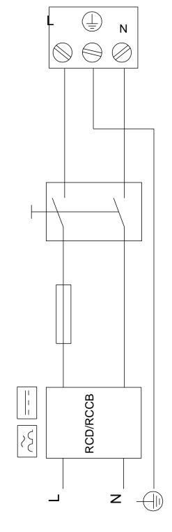
Example of mains-connected motor with mains switch, backup fuse and additional protection
