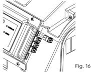
2) Strip 6-8 mm insulation from the end of the connection wire (Max 1.5 mm<sup>2</sup> CSA).
