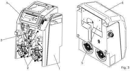
3.12 **Principle of operation:** The pressurisation unit consists of a break tank and one/two peripheral pumps. The break tank is supplied with mains water from either the left or right through a flexible hose connected to a float valve and includes an overflow and weir to maintain an AB air gap in the tank. The unit is connected to the heating/chiller system via another flexible hose which can exit the unit on either the left or right. The pumps are connected to the tank via a rubber connector.
