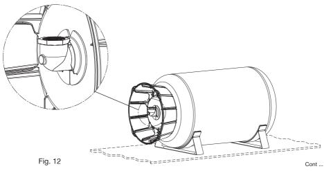
c) Remove the plastic skirt by rotating anti-clockwise to unclip and discard.
