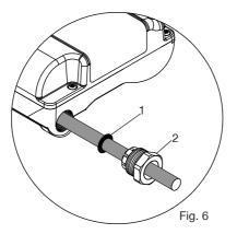
To enable correct assembly of the cable gland the 'O'-ring (Fig. 6 item 1) must be placed over the cable before the clamping insert (Fig. 6 item 2) can be tightened.
