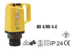
Double insulation in keeping with type of protection class II, splash water protected in keeping with IP 24, double-pole ON/OFF switch and single-pole thermal overcurrent release. 5-m connection cable with plug. Not explosionproof.
