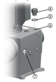
Fig. 12-2: Dosing pump oil inlet
