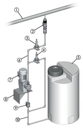
Fig. 8-6: Installation with a back-pressure valve
