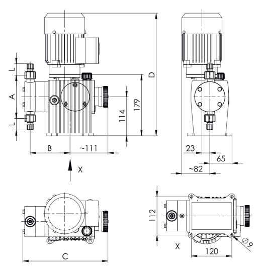
Fig. 6-1: Dimensioned drawings MEMDOS LB 4 – 80 and 150
