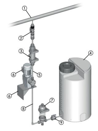
Fig. 8-7: Installation with a pulsation dampener
