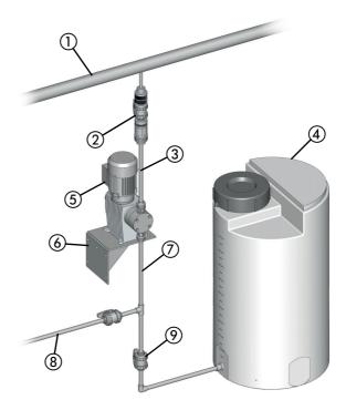
Fig. 8-9: Dosing of suspensions
