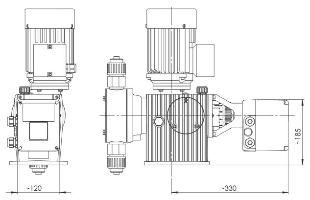
Fig. 6-4: Dimensioned drawings MEMDOS LB 110, 160 – 1010 with electric servomotor
