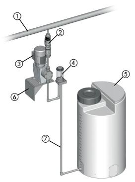
Fig. 8-8: Installation with a priming aid
