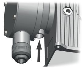
Fig. 8-2: Leakage drain opening
