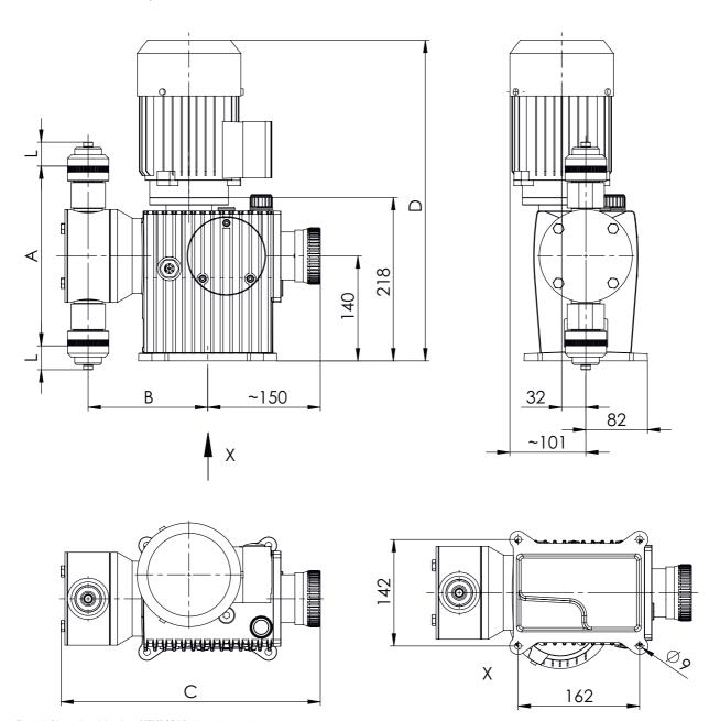
Fig. 6-2: Dimensioned drawings MEMDOS LB 110, 160-1010
