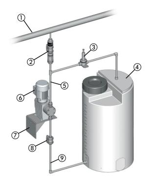
Fig. 8-3: Installation with an injection nozzle
