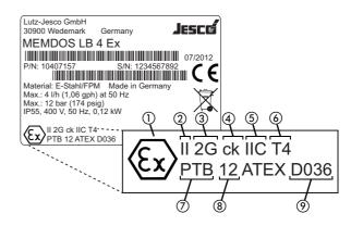
Fig. 4-3: Ratings plate MEMDOS LB with ATEX certificate
