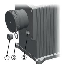
Fig. 12-1: Draining oil on the dosing pump
