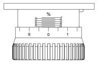
Fig. 10-2: Stroke adjustment scale
