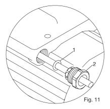
To enable correct assembly of the cable gland the 'O'-ring (Fig. 11 item 1) must be placed over the cable before the clamping insert (Fig. 11 item 2) can be tightened.
