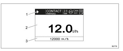
Fig. 5: Construction of continuous display
