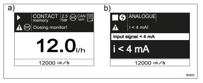
*Fig. 6: a) Continuous display with warning message; b) Continuous display with fault message. Explanation of the symbols in the following tables.*
