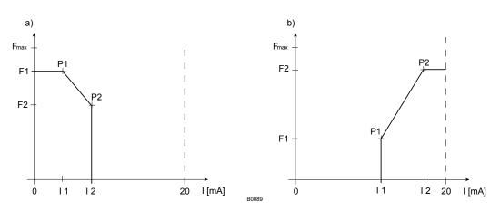
Fig. 32: Frequency-current diagram for a) Lower side band, b) Upper side band
