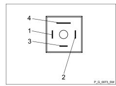
To pin VDE cable Contact Relay "+" Current output 1 yellow "\_" 4 green Current output 3 NC (normally closed) or white Relay NO (normally open) 2 brown C (common) Relay
