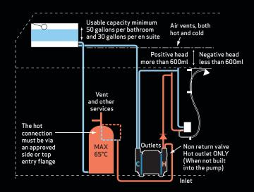
Specifically designed for installation into 'Gravity' systems, the enhanced performance of the **CT Bathroom** range will ensure all outlets within your bathroom perform to their maximum.
