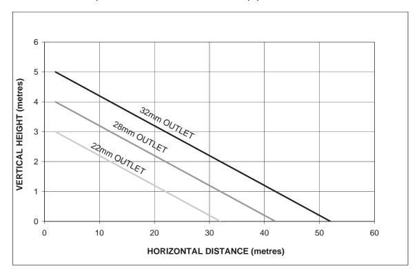
3.23 See diagram above for typical combinations of height and length of discharge when using 32 mm, 22 mm or 28 mm pipework. Do not exceed the guidelines given for pipe diameters.
